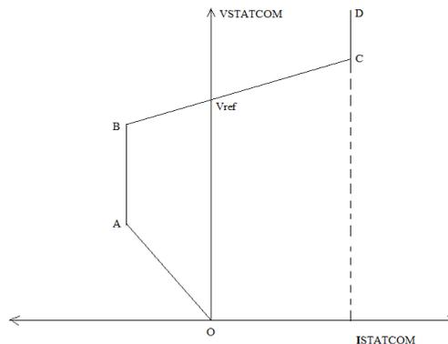
Fig 2: V-I Characteristics of STATCOM
