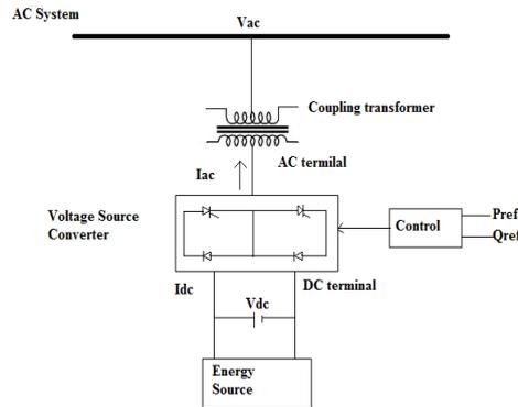
Fig 1: Functional block diagram of STATCOM
